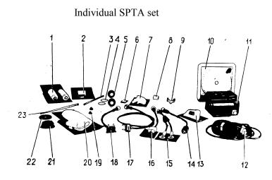
*I* - Rechargeable battery 10D-0, 55C-1; *2* - fuse link VP1-1 1,0A 250 V; 3 - pencil; *4* - sealing ring; *5* - eye shield; *6* - framed lens; *7* - cloth; *8* - eraser; *9* - wrench; *10* - coordinate converter; *11* - charging device; *12* - protection device; *13* - indicating silica gel; *14* through *18* - cable; *19* - membrane; *20*, *21* - cover; *22* - diaphragm; *23* - brush KXOOK No. 7 (made from synthetic fibre)
