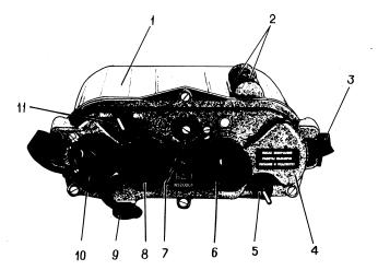
*1* - housing; *2* -MEASURE 1 and MEASURE L buttons; *3* - belt; *4* - panel; *5* - ILLUMINATION toggle switch lever; *6* - Binocular eyepiece; *7* - screw; *8* - indicator eyepiece; *9* -plug MP-1; *10* - battery section cover; *11* - ON-OFF toggle switch lever
