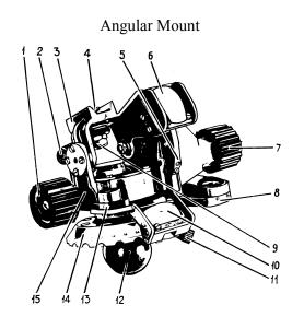
*I* - adjustment knob; 2 - lever; 3 - bracket; 4 - retainer; 5 - scale; 6 - framed lens; 7- adjustment knob; 8 - compass; 9 - nut M8; 10 - framed lens; 11 - knob; 12 - support; 13 - level VK-10; 14 - azimuth circle; 15 - body Fig. 4
