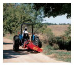
The mounted 451 has an exclusive telescoping yoke that uses tractor power to lift the mower.
