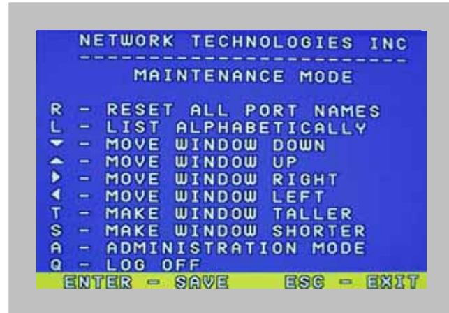
Figure 24- Maintenance Mode screen
