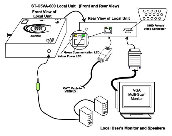
Figure 2- Connect Local User Components to Local Unit
