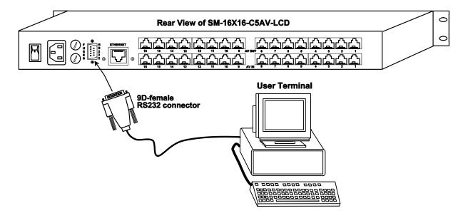
Figure 9- Connect user terminal to VEEMUX
