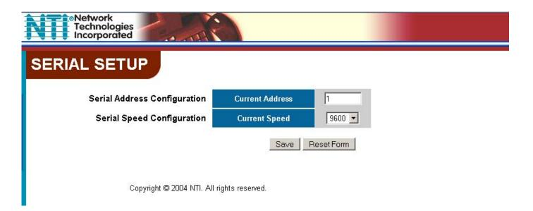
Figure 24- Web interface Serial Setup page
