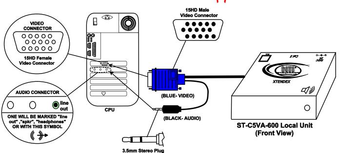
Figure 1- Connect the Local Unit to the CPU
