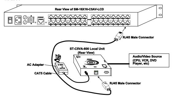
Figure 5- Attach ST-C5VA-600 Local Unit to VEEMUX
