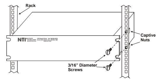
Figure 33- Mount Switch to a Rack
