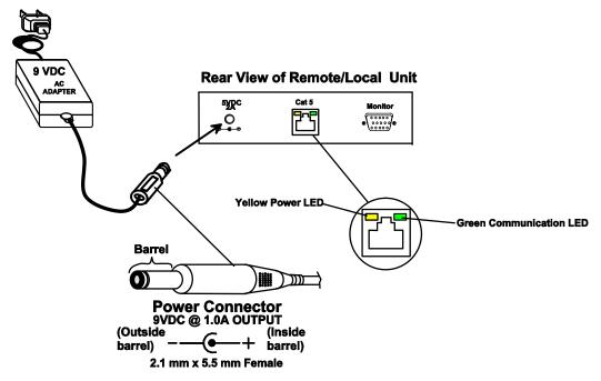
Figure 4- Connect the AC adapters
