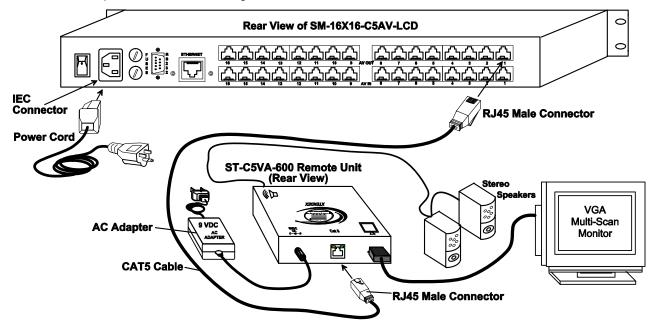
Figure 6- Attach ST-C5VA-600 Remote Unit to VEEMUX
