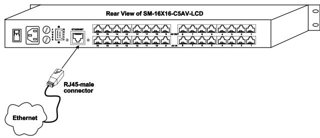
Figure 8- Connect VEEMUX to LAN
