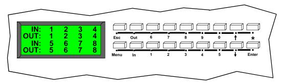
Figure 10- Front panel Interface LCD and keypad
