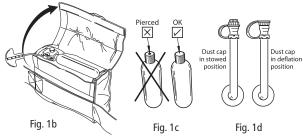
5) Repack the bladder into the pouch (see "Repacking your inflatable PFD"). Make sure the pull tab is hanging freely outside the pouch. If everything checks out according to the preceding instructions, your inflatable PFD is ready for use.
