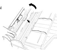
Gently close the scanner cover, making sure both sides are snapped down securely.
