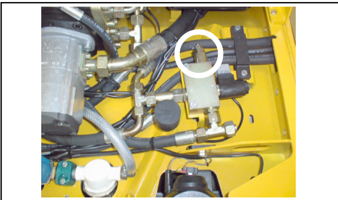
M2 Relief valve when engaging single vibration 1'750 \pm 75 PSI
