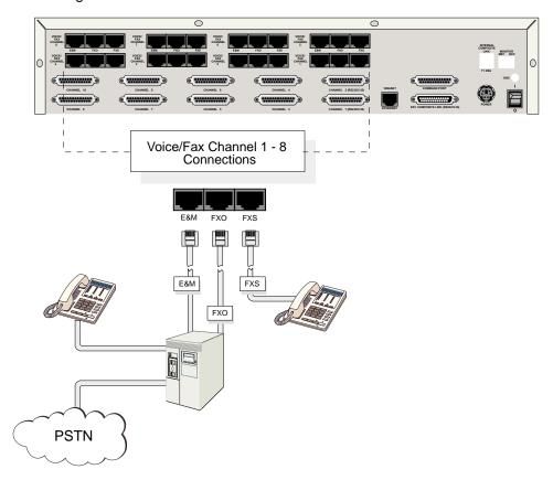
Figure 5. Voice/Fax Cable Connections
