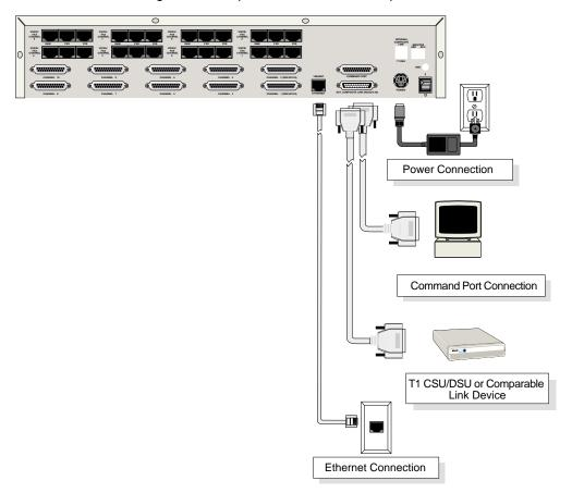
Figure 3. General Cable Connections
