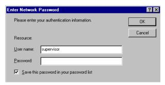
Type **supervisor** in the **User Name** field (no password needed) and click **OK**. The **MultiFRAD 3000 Configuration** screen is displayed.
