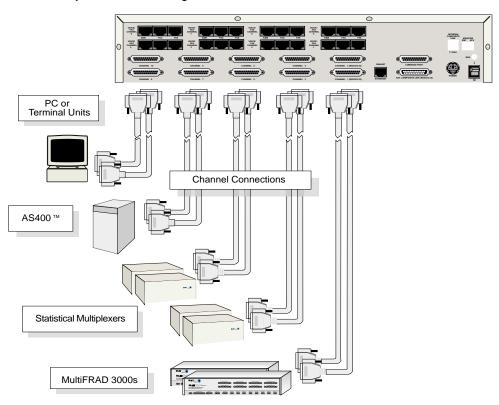
Figure 4. Channel Cable Connections
