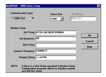
Verify that the **Communication Type** field is set for **COM Port** and the **Select Port** field matches the COM port of your local PC.
