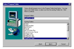
7. After all the program files from both disks are loaded, the Setup dialog box is displayed, enabling you to designate the COM port of your PC that is connected to your MultiFRAD. On the **Select Port** window, click the down arrow and choose the COM port of your PC (COM1-COM4). that is connected to your MultiFRAD.
