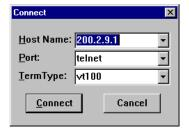
When you enter a valid Host Name (IP address) and click the Connect button, you are immediately connected to the target MultiFRAD and the MultiFRAD Management Menu screen is displayed.
