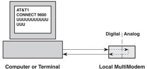
Figure C-1. Local analog loopback test.
