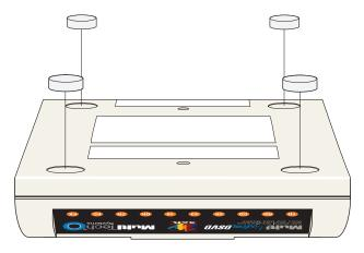
Figure 2-1. Mounting the feet.
