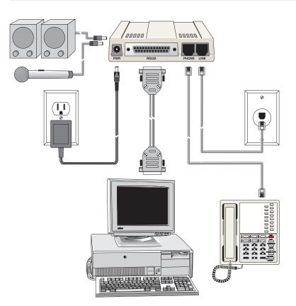
Figure 2-3. Modem connections.
