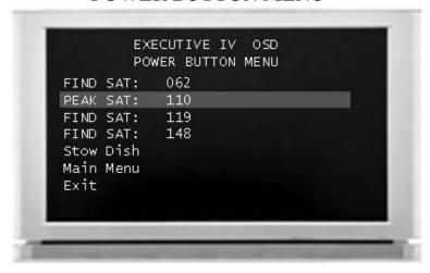
When you're watching TV and you hit the "Power Off" button on your Satellite Receiver, the first screen that will appear will be this Power Button Menu. Here you have the option to move your dish to a different satellite, Stow your Dish, or to go to the Main Menu screen or simply exit.
