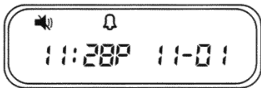
Example of standby screen with alarm enabled
