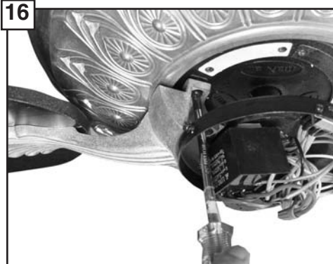
Check the motor for plastic shipping stabilizer tabs, and remove them if they are present. Attach blade assembly to motor using the motor screws and washers provided. Tighten screws securely.
