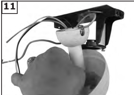
Hang assembled fan from the mounting bracket installed to ceiling in previous step. Make sure the fan is hanging straight. Rotate fan until the tab on the Mounting bracket engages the slot on the Downrod Ball. This must be done to prevent the fan body from rotating when the blades are in motion.
