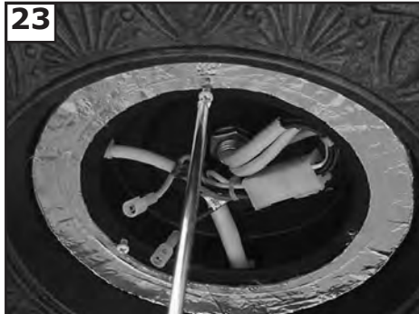
23 Loosen 2 pre installed screws of light kit plate and remove 1 screw. Save removed screw for use later.
