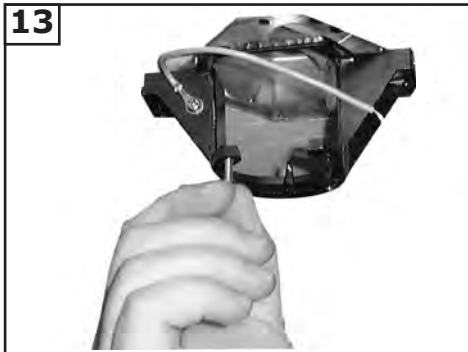
Make sure the studs protruding from the bottom of the Mounting bracket are installed with threads all the way through the bracket.
