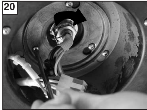
20 Install switch plate by placing over the 2 screws and twisting into place. Install screw removed and tighten all 3 screws securely.
