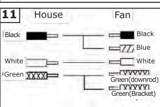
For pullchain controls, follow diagram above. Make sure that all exposed wiring is secured inside wire nuts. Note: Wires from house may vary in color and may not include ground wire. After wiring is conplete, gently push wires into junction box with wire nuts pointing upward. Refer to point 3 of safety tips.
