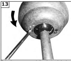
Raise the canopy up and align the two holes in the canopy with the two holes in the hanger bracket. Secure with two screws provided.
