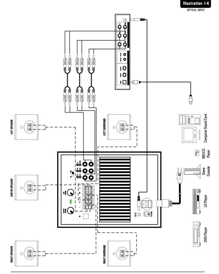
Using the **Optical Input** on the S4 MidiLand 8200 v2.0, users may use this system with wide variety of sound sources equipped with an optical connector for sound output. The **Optical Input** along with **Coaxial 1** and **Coaxial 2** can be connector simultaneously. User may select to use either the Optical Input, Coaxial 1 or Coaxial 2 by pressing the input button on the remote control.
