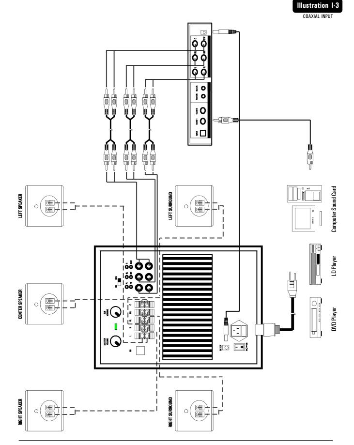
Using the **Coaxial Input** setup on the S4 MidiLand 8200 v2.0, users may use this system with a wide variety of sound sources which is equipped with coaxial (RCA) connector for sound output. Up to two different types of sound sources equipped with coaxial output may be connected to the ADS 4000 through the use of **Coaxial 1** and **Coaxial 2** connector simultaneously. User may select to use either Coaxial 1 or Coaxial 2 by pressing the input button on the remote control.
