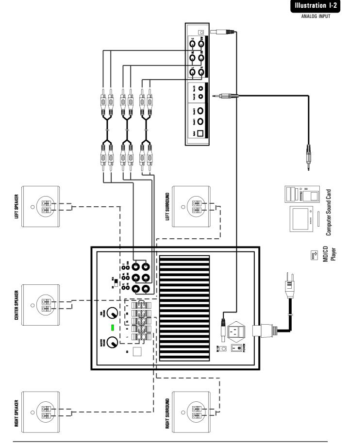
By using the **Front Analog Input** on the S4 MidiLand 8200 v2.0, users may use this system with a wide variety of sound sources. Some sound sources may require different analog cables other than the cables supplied with this system. Please refer to your sound source manual for the correct type of cable(s) needed, which can be purchased at your local electronic/audio stores.
