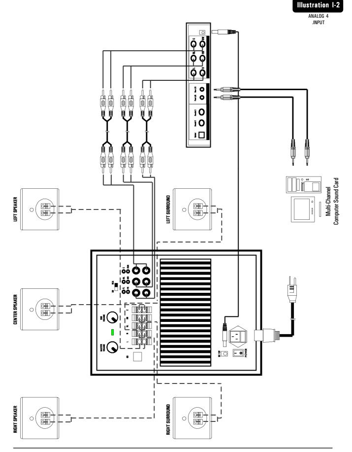
By using the **Front and Rear Analog Inputs** on the S4 MidiLand 8200 v2.0, users may use this system with a multi-channel sound card to expericence 4.1 channel surround sound effect in games as well as in music. Using this setup, only the front, rear and subwoofer will be the default speakers to produce sound. Center channel speaker will remain idle. Please refer to your sound card's manual for the correct output jack location.
