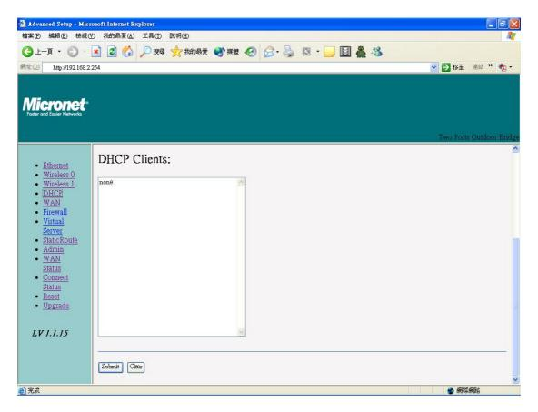
**DHCP Server Control: Dynamic Host Configuration Protocol** assigns dynamic IP addresses to devices on the network. This protocol simplifies network management and allows new wireless devices to receive IP addresses automatically without the need to manually assign new IP addresses.
