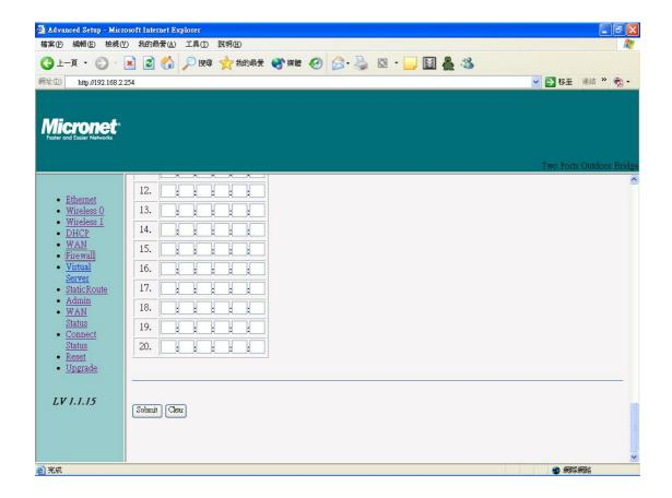
In Firewall IP Rules fields you can define 20 IP rules to deny or pass networking which fit the rules.
