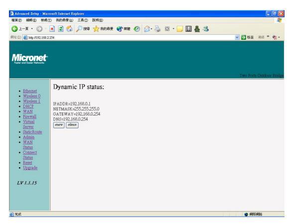
When WAN setting is **Dynamic IP** or **PPPoE** click WAN Status will show current IP status. You can click **renew** or **release** to renew or release IP at **Dynamic IP** setting, and click **disconnect** or **connect** to disconnect or
