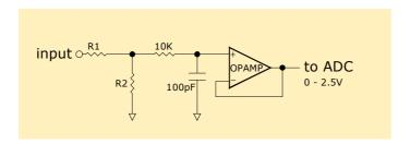
The analogue inputs on PV1800 are factory configured by choosing proper values for R1 and R2. In the table the values are shown for the different models. The input resistance is  $1M\Omega$  on all voltage input channels. The software interface is explained in section *PV-1800 register interface*.
