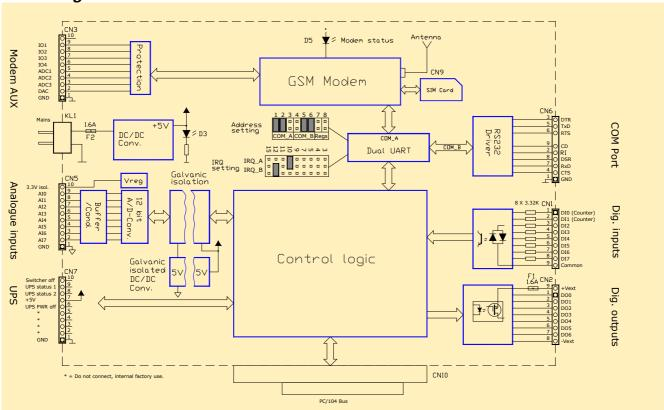
The PV-1800 has an onboard DC/DC converter that converts the incoming mains (+8-35V DC) to +5V. This power supply delivers +5V, up to 4A, to the PV-1800 and to the PC/104 bus. A mains fuse F2 (1.6A) is placed on the rear side of the PCB, near KL1. In PV-1800A versions, where the DC/DC-converter is omitted, the module receives its power from the PC/104 bus.
