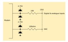
These I/Os are operated by AT commands in the modem.
