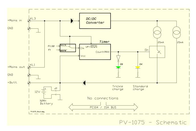
Micronix PV-1075 is a PC/104 module that contains a NiMH battery pack, a timer controlled charger and four connectors.
