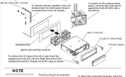
Before mounting and operating the CD player, remove the metal mounting sleeve illustrated by the arrows.
