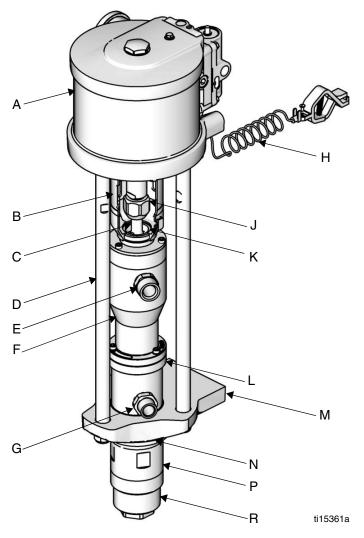
Fig. 1. Component Identification
