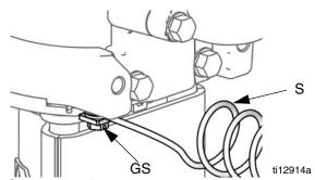
Fig. 4. Ground the Pump.
