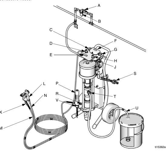
Fig. 3: Typical Cart-Mount Installation
