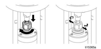
Fig. 8. Remove coupling collars.
