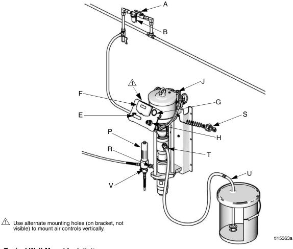
Fig. 2: Typical Wall-Mount Installation
