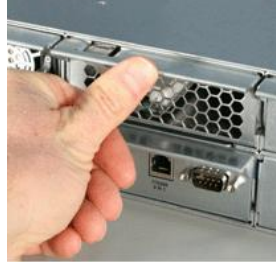
Figure 19: Replacing the cooling unit into enclosure
