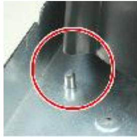
Figure 15: Positioning the blower onto mounting pins
