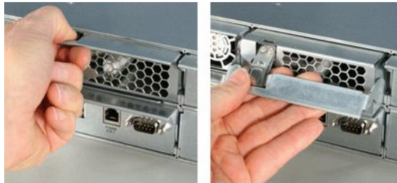
Figure 17: Removing the cooling unit from enclosure
