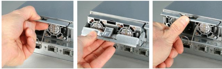
Figure 11: Replacing a Power Supply
