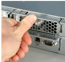
Figure 16: Locking the cooling unit handle
