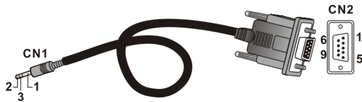
Figure C-19: Adapter Cable for COM1 - Connector Pinouts
