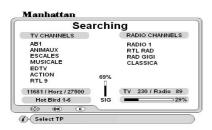
When searching, this page will show the TV and Radio channels it found. After completing the index, the positioner will move the antenna to the first satellite.
