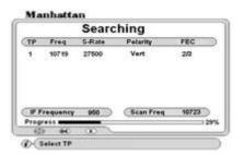
Shows serial number of TP, Frequency, Symbol Rate (S/R), Polarity and FEC.
