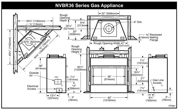
Fig. 1 NVBR36 Series specification and framing dimensions.
