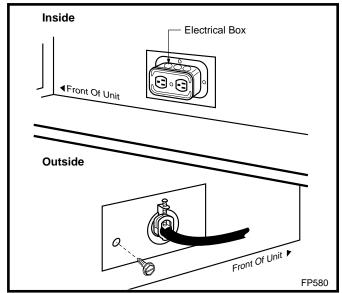
**Fig. 11** Junction box (EB-1) hook-up.
