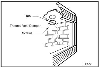
Fig. 21 Attach the thermal vent damper.
