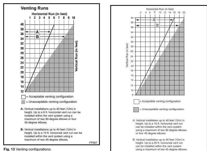
Fig. 13 Venting configurations.
