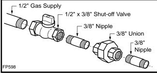
Fig. 8 Typical gas supply installation.
