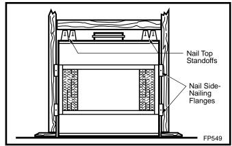
Fig. 6 Adjustable drywall strip (nailing flange).
