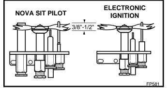
Fig. 20 Proper pilot flame height.
