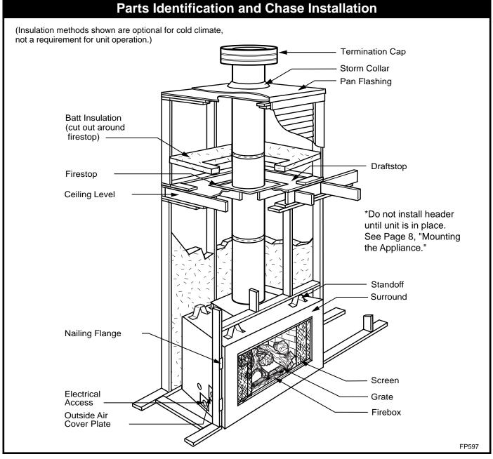
Fig. 7 Parts identification and system installation.
