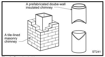
Fig. 3 Standard chimney types.
