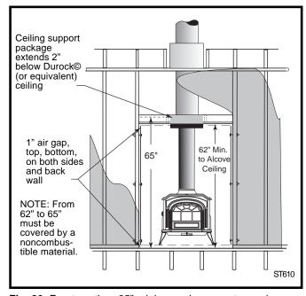
**Fig. 26** Front section: 65" minimum clearance to combustibles on front face. Combustible facing may overlap metal studs by only 1". It should not extend below the height of the noncombustible ceiling.
