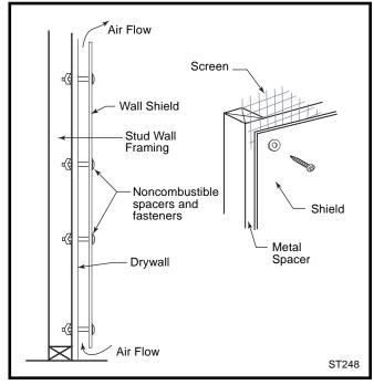
Fig. 13 Approved wall shield construction.
