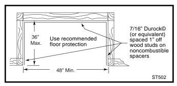
Fig. 24 Floor plan. Sheetrock on front face butts to Durock© (or equivalent) alcove lining.
