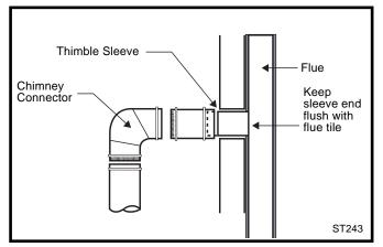
**Fig. 5** The thimble, made of either cermaic or metal, must be cemented securely in place.
