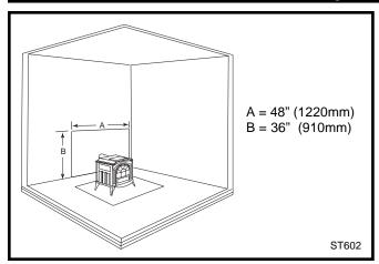
**Fig. 16** A rear-exit stove with reduced rear wall clearance only.
