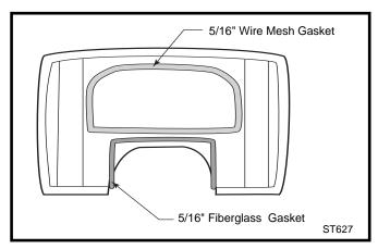
**Fig. 40** A 5/16" wire mesh gasket seals the griddle to the stove top. The flue collar is sealed with a 5/16" fiberglass gasket.
