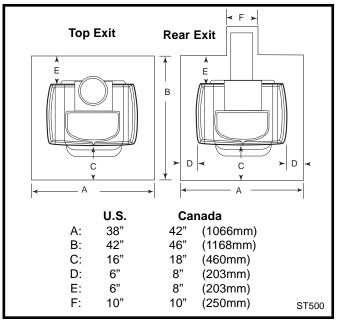
Fig. 11 Required floor protector dimensions.
