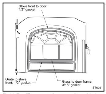
**Fig. 39** Two different gasekt sizes are used to seal the front door.
