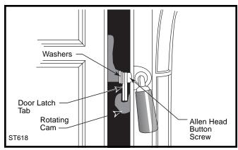
**Fig. 34** The front door seal can be adjusted simply by adding or removing washers.
