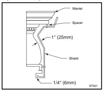
Fig. 14 A custom-formed mantel shield.
