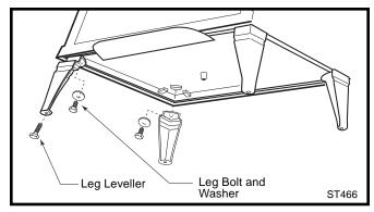
Fig. 26a Attach stove legs and leg levellers.
