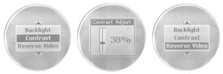
Contrast is highlighted on the Screen menu (left). The Contrast Adjust window (center). Reverse Video highlighted on Screen menu (right).
