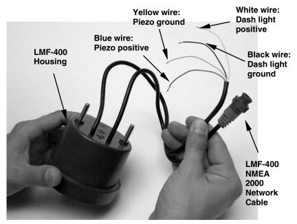
LMF-400 with power cable wiring and NMEA 2000 Cable Connection. Connecting to a NMEA 2000 Network
