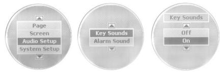
Audio Setup highlighted on the basic menu (left). Audio Setup menu (center) with Key Sounds menu (right).
