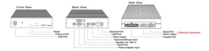
As it's a fan-less computer, adequate ventilation is required to ensure normal operation. Allow at least 6 inches of space from the top of the unit and 3 inches from the sides to allow proper ventilation.
