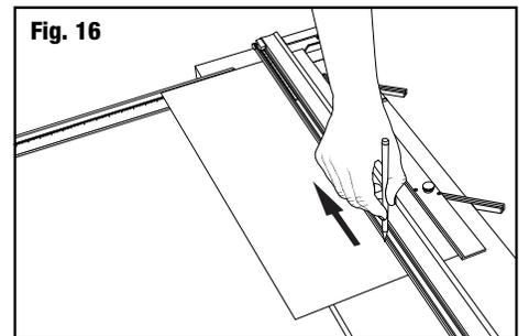
6. Attach the 702 Bevel Cutter to the Guide Rail by fitting the black nylon guides over the raised edge of the channel.
