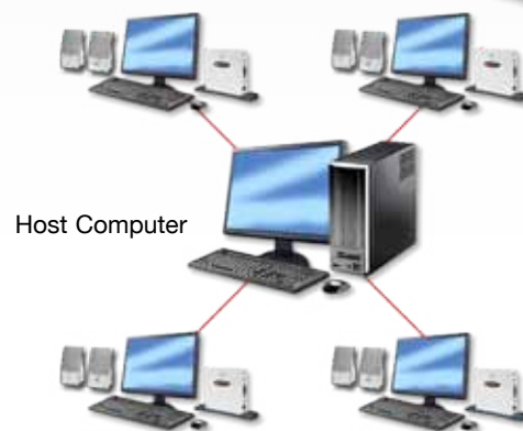
Up to 10 User Clients can each be connected to the host using a single USB cable
