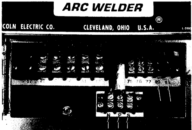
Terminal Strip of DC-600 (Codes Below 8200 only).
