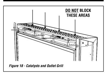
It is recommended that the catalysts are inspected for signs of damage and dirt during routine servicing procedures. The expected life of the catalysts is in excess of 11,000 hours (10 years of normal use). After this time the catalyst should be replaced.
