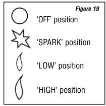
The control knob is located on the lower right hand side of the outer case. It is of a spherical design and is marked as shown in Figure 19.
