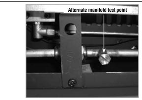
Figure 8 - Alternate Test Point
