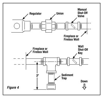
An ANSI approved manual shut-off valve and union must be installed upstream of the heater within the fireplace cavity when rigid pipe is used. Ensure that a sediment trap is installed upstream of the heater (*Figure 4*) within the structure's piping system to prevent moisture and contaminants from passing through the pipe to the heater controls and burner. Failure to do so could prevent the heater from operating reliably.
