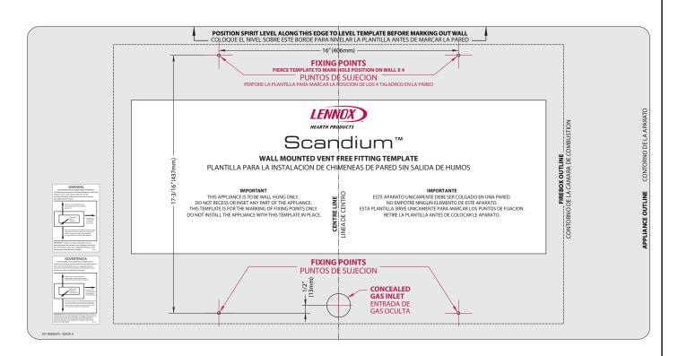
Figure 2 - Wall Fixing Template
