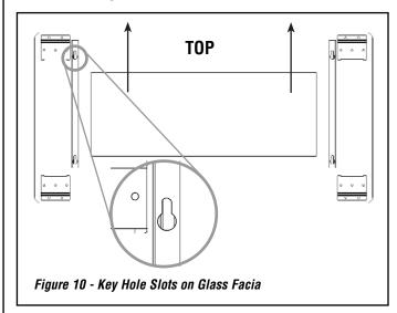
Slide on the side pieces ensuring that the grill fixing holes (shown) are aligned towards the top of the glass facia (as shown in *Figure 11*).
