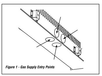
Non-concealed gas connections may be made using the entry points on the base of the firebox. A concealed gas connection may be made using the knockout hole in the center back of the firebox. Select the most appropriate entry point and knock out the relevant hole.
