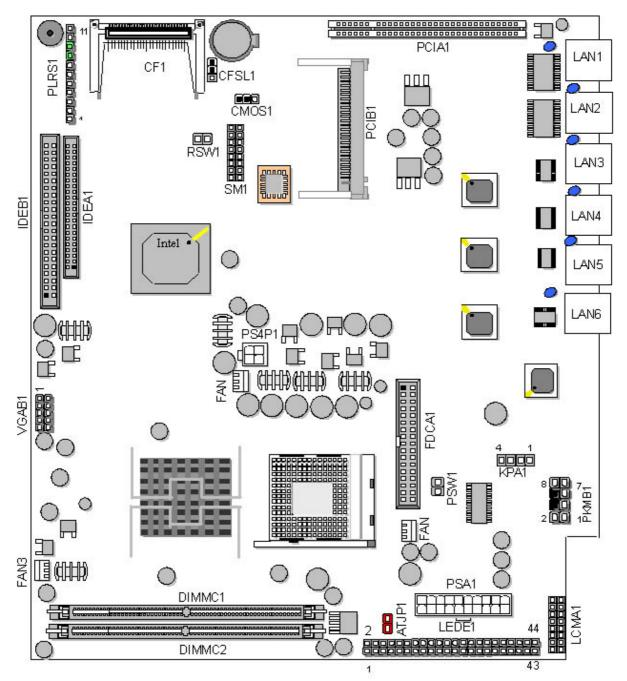
Figure 3 - MB-X71 Jumpers and Connectors
