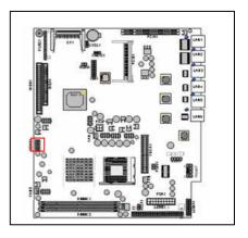
IDEA1 : IDE Interface Connector ( 44Pin 2.0mm Pitch Header )
