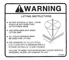
Figure J WARNING, LIFTING INSTRUCTIONS Part Number 172-820 1 Required ALL MODELS
