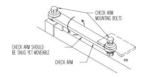
Vertical check bolts must not be tight (and should be free to rotate by hand) and need not less than 1/16" and no more than 3/32" free play when properly adjusted on level ground.
