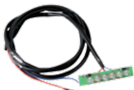
Led replacement for Extreme tail-light Ricambio led portatarga Extreme R-LEDRS000006
