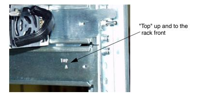
3. Adjust the length of the rail to fit between the channels in the rack/cabinet.
