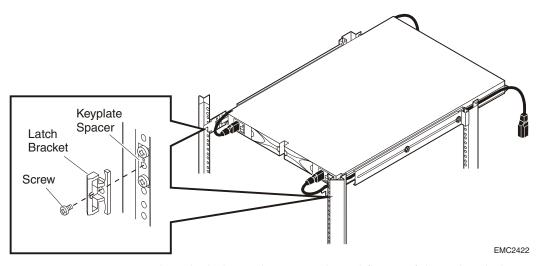
8. Align the holes in the rear, u-shaped flange of the rail with the holes in the rear inside channel.
