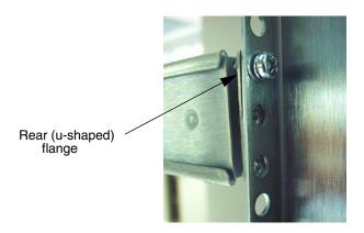
9. Secure the rail to a round-hole rear channel with 2 M5 x 12 mm pan-head screws (see the table on page 3), or secure the rail to a square-hole rear channel with 2 square-hole washers and M5 x 16 mm flat-head screws (see the table on page 3). Leave the screws finger-tight, and tighten them after the switch is installed. See the figures below.
