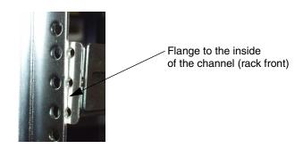
6. Secure the rail to a round-hole channel with 2 M5  $\times$  12 mm pan-head screws (see the table on page 3), or secure the rail to a square-hole channel with 2 square-hole washers and
