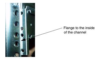
6. If you are installing a switch in a 39U cabinet, secure the rail to a round-hole channel with one M5 x 12 mm pan-head screws and one #10 flat washer and ball stud (see the table on page 3), or secure the rail to a square-hole channel with one square-hole washer and M5 x 16 mm screw and one #10 flat washer and ball stud (see the table on page 3). Leave the screw and ball stud finger-tight. Tighten them after the switch is installed. See the figures below.
