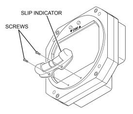
Figure 4.1, Inclinometer Installation
