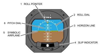
Figure 1.2, Typical Display Features
