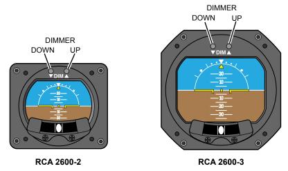
Figure 3.1, Dimming Controls
