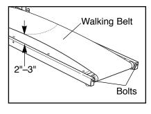
Using the allen wrench, turn both rear roller adjustment bolts counterclockwise 1/4 of a turn. When the tension of the walking belt is correct, you should be able to lift each side of the walking belt 2 to 3 inches. Walk on the treadmill for a few minutes. Repeat until the walking belt is properly tightened. Be careful to keep the walking belt centered.
