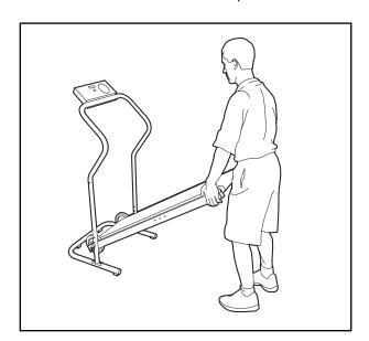
2. Move your left hand to the position shown and hold the treadmill firmly. Using your right hand, insert the Short Pin (4) through the Handrail (6) and the Frame (32) as far as it will go.
