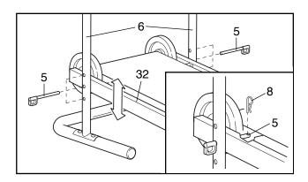
the Frame, align the holes in the Frame with one of the three sets of holes in the Handrail (6), and reinsert the Long Pins. **Make sure both Long Pins are at the same level.** Refer to the inset drawing. Insert a Cotter Pin (8) into the hole in each Long Pin. **Make sure that the Long Pins are fully inserted into the holes.**
