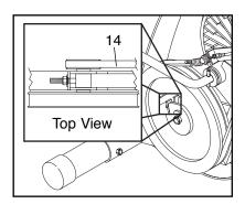
If the Drive Belt (14) is properly adjusted, reattach the side shields and pedals. If the Belt needs to be adjusted, loosen the Nylon Locknut (7) on the left side of the Flywheel
