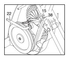
Strap, **fully** close the Strap Clamp. Turn the Crank (22) for a moment to make sure that there is not too much resistance. When the Resistance Strap is properly adjusted, reattach the left side shield and pedal.
