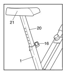
remove the Seat Pin (16). Align one of the holes in the Seat Post (20) with the hole in the Frame (1). Insert the Seat Pin into the Frame and the Seat Post. Caution: Make sure to insert the Seat Pin through one of the holes in the Seat Post; do not insert the Seat Pin under the Seat Post. In addition, make sure that the Seat Pin is inserted into the front of the Frame and the Seat Post as shown above.
