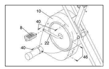
ed. Using an adjustable wrench, turn the Left Pedal (8) clockwise and remove it from the Crank (22). Remove the three Side Shield Screws (40) and the two M4 x 16mm Screws (46) from the Left Side Shield. Make sure that the arm of the Crank is in the position shown in the drawing above. Carefully slide the Left Side Shield forward off the arm of the Crank and remove it.
