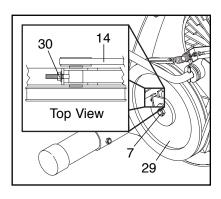
(29). To tighten the Belt, turn the M10 Nut (30) clockwise; to loosen the Belt, turn the M10 Nut counterclockwise. Make sure that the Flywheel is straight and tighten the Nylon Locknut (7). Reattach the side shields and pedals.
