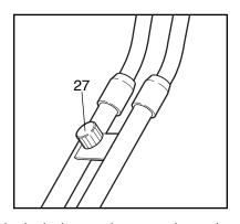
the Resistance Knob clockwise; to decrease the resistance, turn the Resistance Knob counterclockwise.
