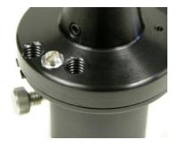
Note: The QuickPan IV rotator uses a stainless steel ball plunger that is different from the plastic nosed plunger on the QuickPan III. Be sure to use only the stainless steel ball plungers (available from Kaidan) on the QuickPan IV rotators. 4) The new Detent Disc is installed by pushing it into the recessed area in the top of the Rotator Hub as shown at left.
