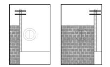
Looking through the viewfinder align a close object (brick wall) with a faraway object (telephone pole). As you rotate the camera from side-to-side there should be no relative movement between the two objects as shown to the right.
