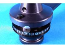
3) Depress the brass plunger and push up on the Indexing Ring until the brass plunger pops into the plunger hole and the pin slides into the notch.
