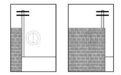
If, as shown above, the two objects move with respect to one and another in the viewinder, slide the camera fore or aft in order to eliminate this movement. Here, the telephone pole has moved behind the brick wall. move with respect to each other as you rotate the pan from left to right. Slide the camera to the front or rear as required to eliminate this relative movement.
