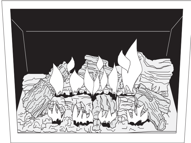
Figure 26. Proper flame pattern.
