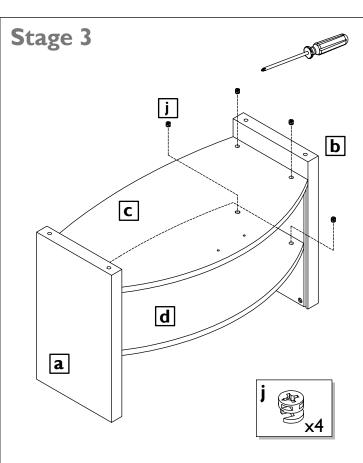
Position shelves **C** and **d** onto metal dowels.
