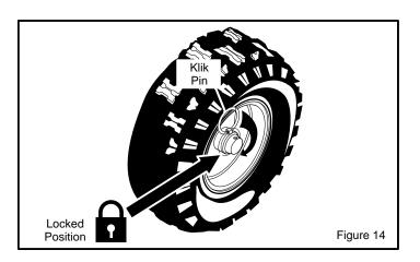
For ease of maneuverability when lighter conditions prevail, remove klick pin from wheel locked position and insert into single wheel drive (unlocked) position (Figure 15). Make sure that the klick pin is in the single wheel drive position of the axle only and not through the locked position.
