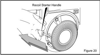
As engine warms up move choke lever to "1/2 choke" position. When engine does not run smoothly, move choke lever to the off position.
