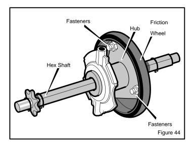
13. Install the **hex shaft** and **bearings** with the four bolts removed earlier (see Figure 45).
