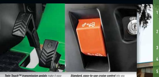
**Twin Touch™ transmission pedals** make it easy to switch from forward to reverse, and let you rest your heel on the platform the whole time you drive.
