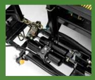
BREAKAWAY BOOMS Spray around trees with confidence. Standard bi-directional breakaway protects boom if object is struck while moving forward or backward.
