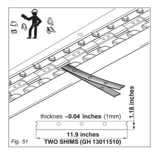
To restore the correct tolerance:
