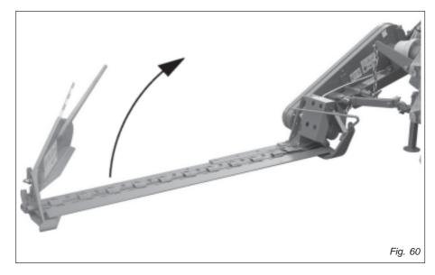
For transport, adjust and fix the chains of the side lifting arms of the tractor; lift the mowing bar (Fig. 60); secure it with the hooking tie rod (A, Fig. 61); slide in the safety hook (B, Fig. 61); cover the cutting blades and the outer mowing bar support with the guards provided (Fig. 62); lift the implement; put the hydraulic lifting command lever in the locked position.
