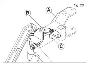
Connections between frame joint and stop bushing for the movement of the mowing bar.
