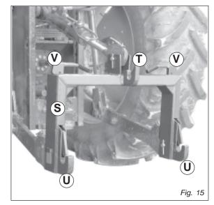
3) Raise the Quick Coupler (S, Fig. 15) and make sure that sickle bar hitch is in the right position (Z, Fig. 16).
