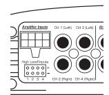
If you wish to send four discrete channels into the e4300, simply use all four inputs (channels | & 2 and channels 3 & 4) and set the "CH 3&4 Input From" switch to "Discrete".
