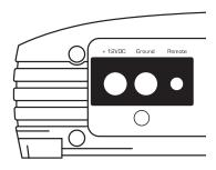
The e4300's "+12 VDC" and "Ground" connections are designed to accept 8 AWG - 4 AWG power wire. 8 AWG is a minimum power wire size for this amplifier.
