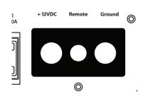
The J2-320.4's "+12VDC" and "Ground" connections are designed to accept 4 AWG power wire. 4 AWG is a minimum power wire size for this amplifier.
