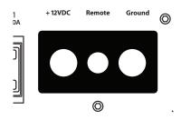
The amplifier will turn on when +12V is present at its "**Remote**" input and turn off when +12V is switched off. If a source unit does not have a dedicated remote turn-on output, the amplifier's turn-on lead can be connected to +12V via a switch that derives power from an ignition-switched circuit.
