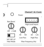
1) "Filter Mode" Control: The J2-320.4 employs a 12dB per octave filter for each pair of channels (one filter for channels 1&2 and another filter for channels 3&4). Each of these filters can be configured independently into one of two filter types or defeated completely by way of the three-position "Filter Mode" switches:
