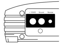
The e1800D's "+12VDC" and "Ground" connections are designed to accept 4 AWG power wire. **4 AWG is a minimum power wire size** for this amplifier.
